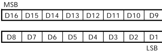
D1-D16 represent digital input status for channels 1 through 16. AX5410P registers can be accessed easily through direct I/O instructions, using whatever application language available (i.e., Assembly, Basic, Pascal, C, etc.).
