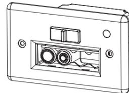
1. Open the battery door by pressing the two tabs located on the door.
