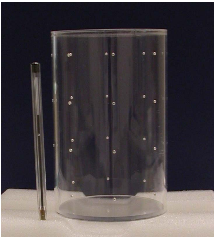
Fig. 11 Exxim's 100mm plastic phantom with metal beads.
