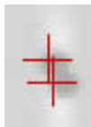
Fig. 15 Bead shadows are overlapped. Please do not use such projections to calibrate your scanner.
