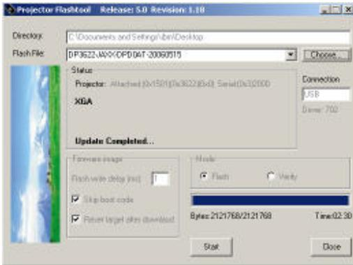
**Note:** After the new firmware is upgraded, the Flash-Tool will perform the final validation. The dialog shows the checksum with a verification message!
