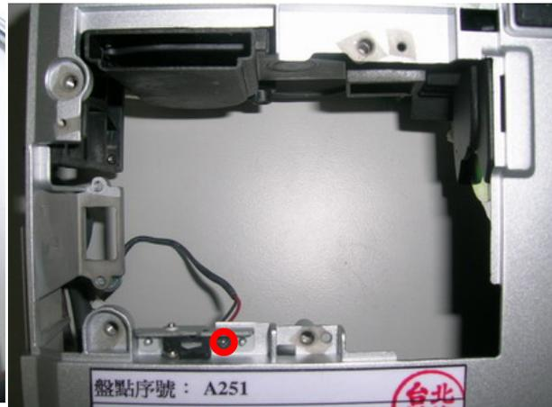
Remove the screw and replace the inter-lock switch board (S23).
