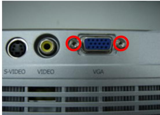
Remove the two hexagonal screws.
