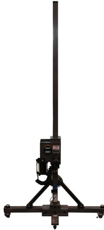
7-TR Tripod Positioner with Pneumatic Polarization Option
