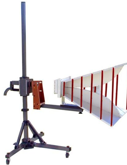
*Model 3106B shown mounted onto 7-TR/POL-M
