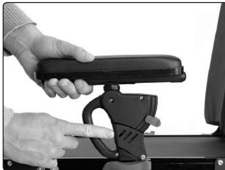
Adjustment of arm rest height
