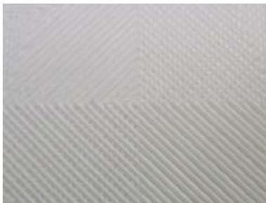
High (50%) - For the object which should be durable or will be used as functional mechanical part, it is suggested to select higher density.
