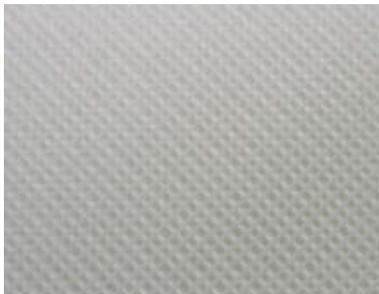
Medium (30%) - The selection gives higher strength to the structure than low density. To print an object for mechanical purpose, it is advised to set the density to 30% or above.
