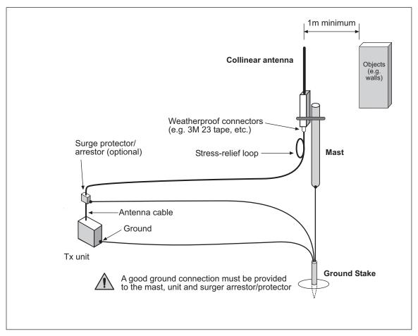
The antenna must be be installed above all local obstructions
