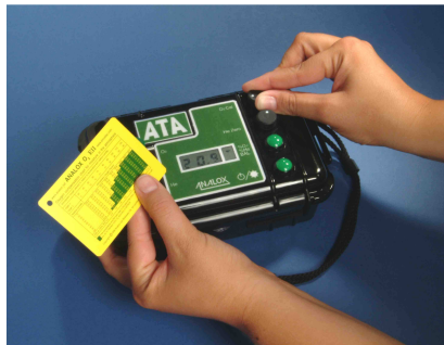
O 2 calibration in clean air
