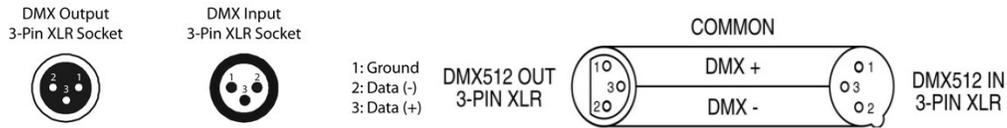
For installations where the DMX cable has to run a long distance, or is in an electrically noisy environment, it is recommended to use a DMX terminator. This helps in preventing corruption of the digital control signal by electrical noise. The DMX terminator is simply an XLR plug with a 120  $\Omega$  resistor connected between pins 2 and 3, which is then plugged into the output XLR socket of the last fixture in the chain. Please see illustrations below.
