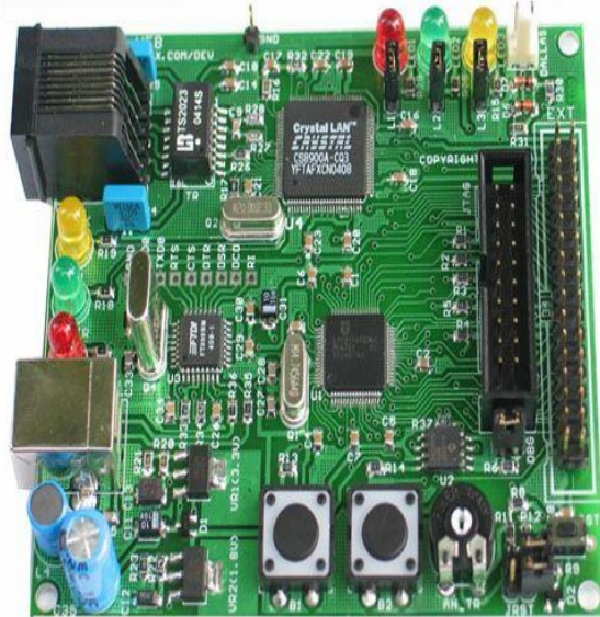
Fig. 3 LPC2129 ARM development board
