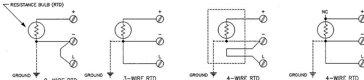
**RTD TRANSMITTER INPUT CONNECTIONS**
