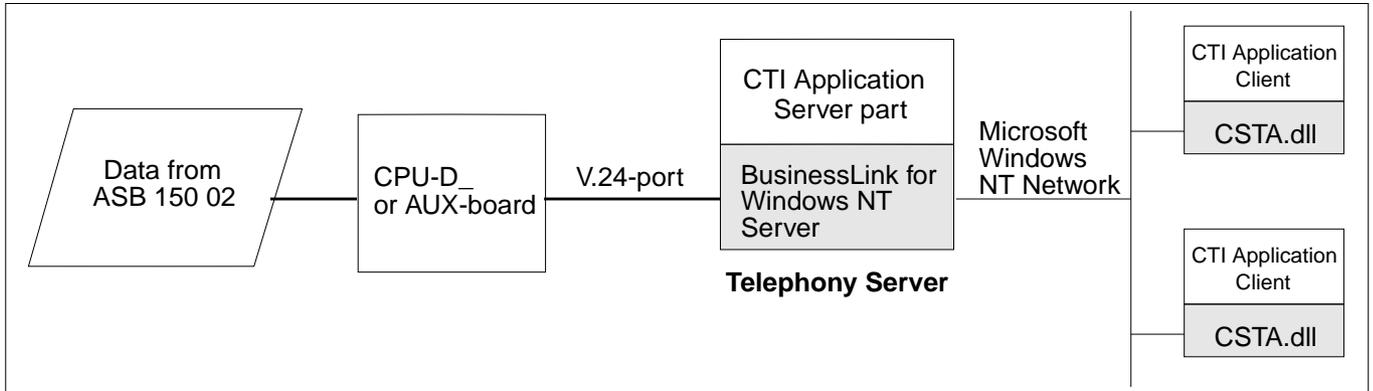
**NOTE:** For BusinessLink for Windows NT a FECU must be plugged into specific port on CPU-D\_.
