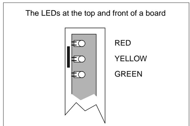
When the start-up is successfully completed, all LEDs in the figure above are turned off. Proceed to section 4 on page 5.
