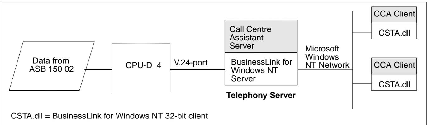
**NOTE:** For BusinessLink for Windows NT a FECU (minimum Package 6: KDUBS 103 0x / 6) must be plugged to specific port on CPU-D\_4.
