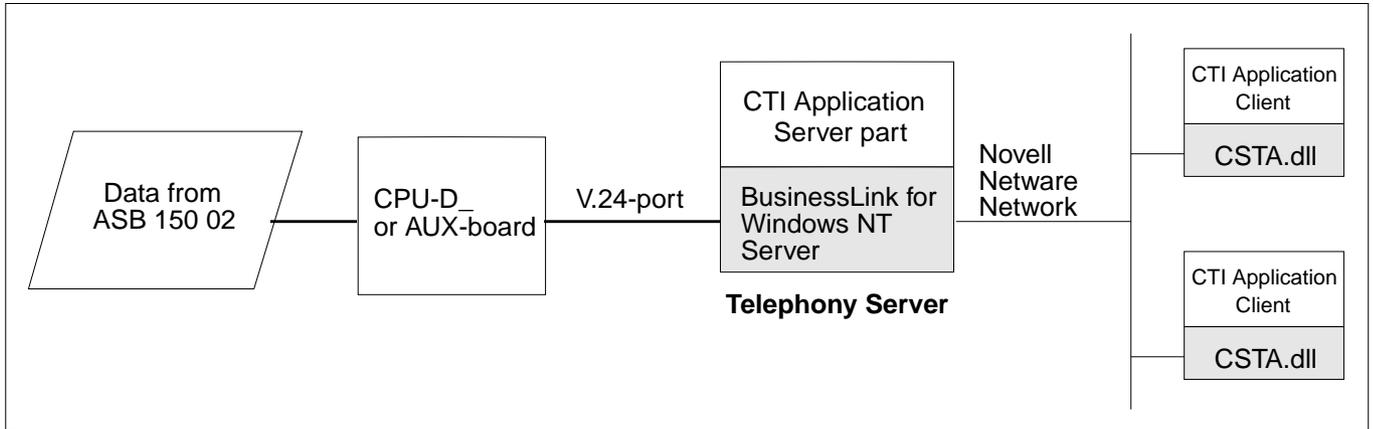
**NOTE:** For BusinessLink for Windows NT a FECU must be plugged into specific port on CPU-D\_.
