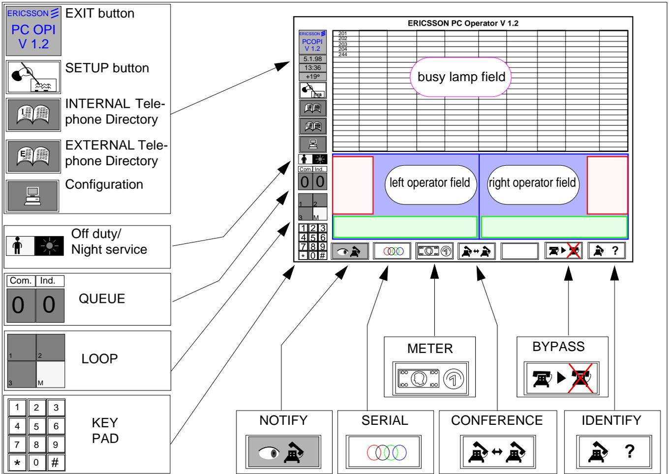
Figure 2 PC OPERATOR Main Screen
