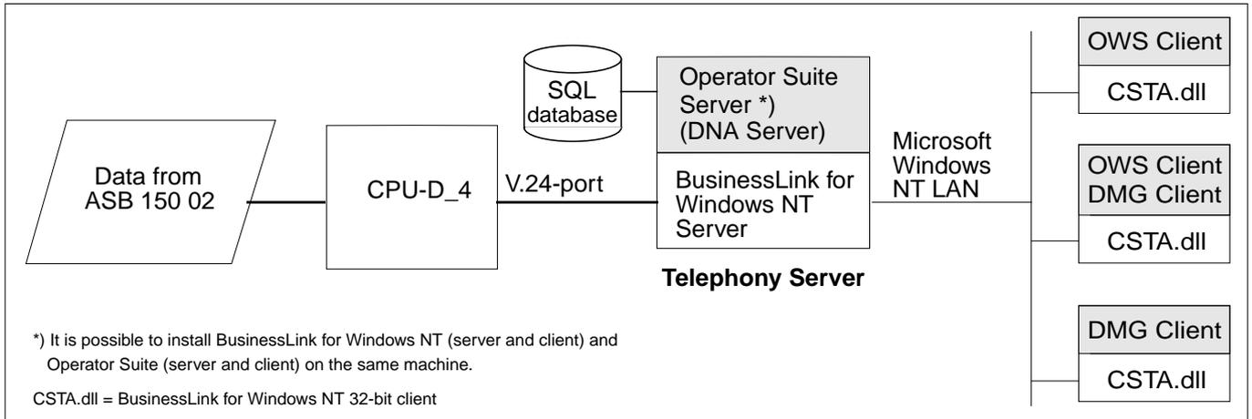
**NOTE:** For Operator Suite a FECU (minimum Package 1: KDUBS 103 0x / 1) must be plugged to specific port on CPU-D\_4.
