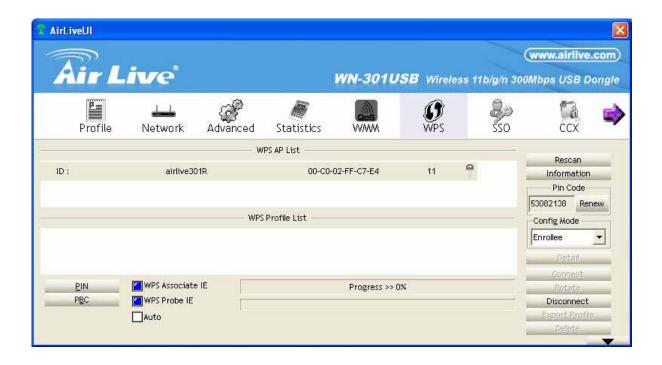
The adapter supports WPS (Wi-Fi Protected Setup), allowing connection to wireless APs without complicated procedures. Two WPS configuration methods are available: PBC (push-button configuration) and PIN.
