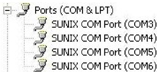
(3) You also can check SUNIX DevicePort® box and COM/LPT port mapping status over **SUNIX DevicePort® Control Center** by executing **dp icon** on the windows desktop system tray.
