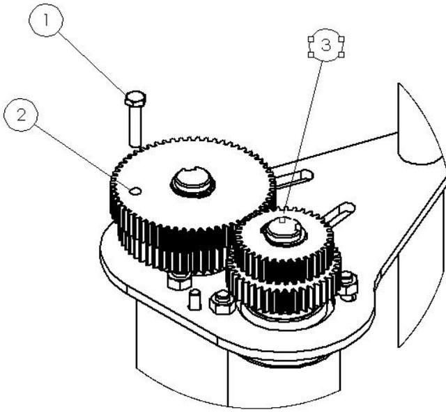
If the bolt (1) is fitted in position 2, the top set of gears provide the stretch (55%).
