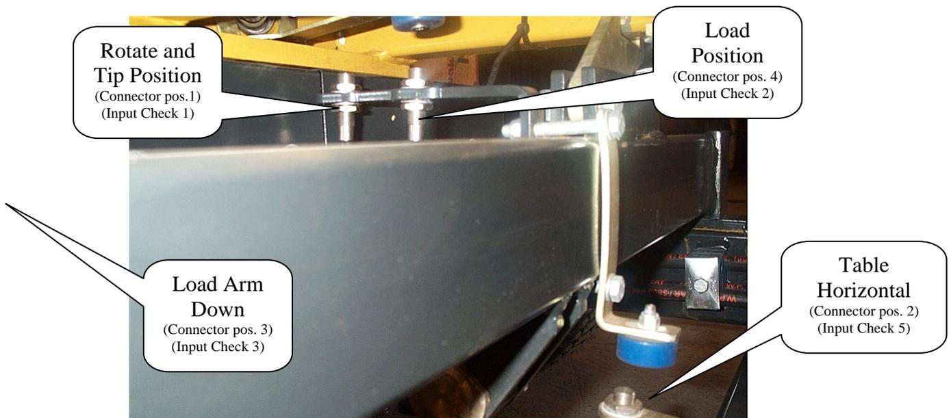
The status of the sensor inputs to the controller can be checked by pressing and holding the down button on the 4 way menu button.
