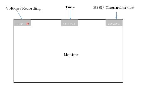
**Voltage indicator:** input voltage value is displayed; Display from 6.5V to 26.5V. **Recording indicator:** a red "R" flashes when DVR is working in the background.
