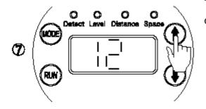
The option No. is displayed. Press Up button to check the option value
