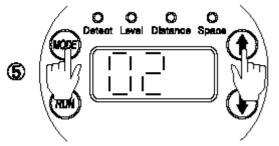
The next option No. is displayed. Press Mode and Up buttons simultaneously to move into next option group.
