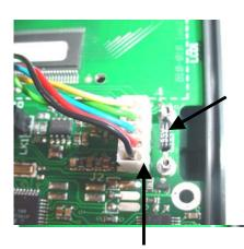
Shunt Calibration Resistor
