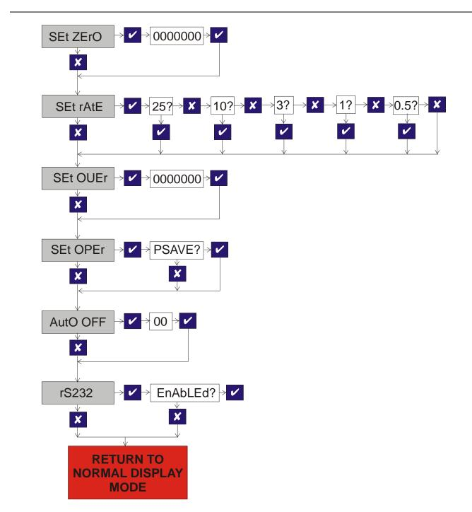
A Calibration Menu, which is used to calibrate each of the two ranges with independent scales, as well as setting the display resolution for each range.
