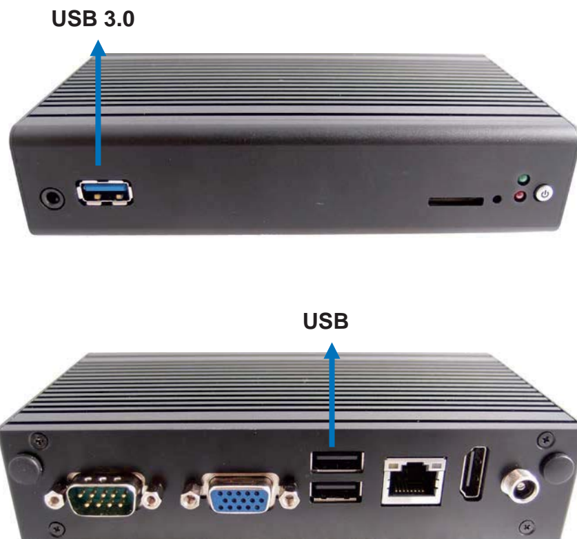
Figure 5 Connect USB mouse & keyboard
