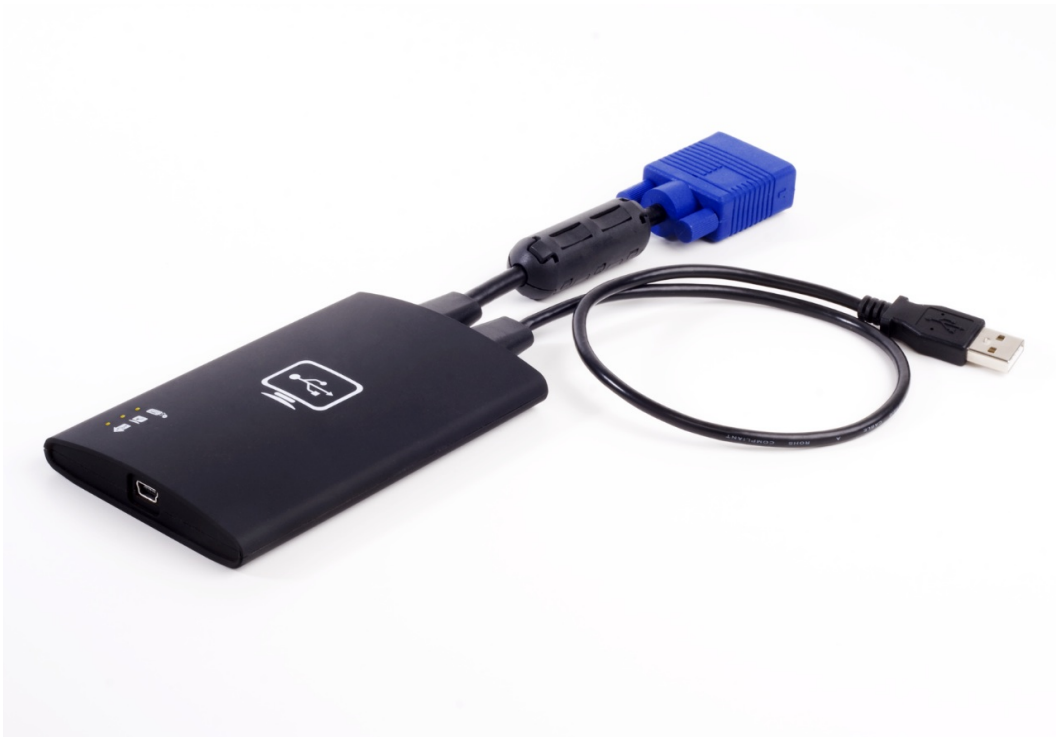
Figure 1: Photo of the USB Laptop Console main unit, with attached cables.
