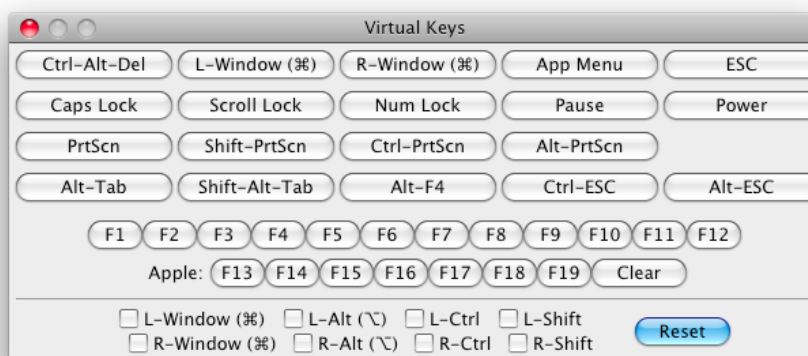
Figure 4.5: This window allows you to send special key sequences to the attached host, without actually typing them.
