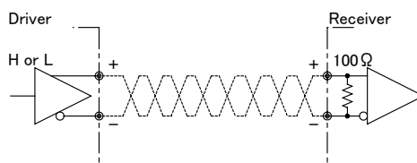
Figure 3-3-2 Circuit of LVDS
