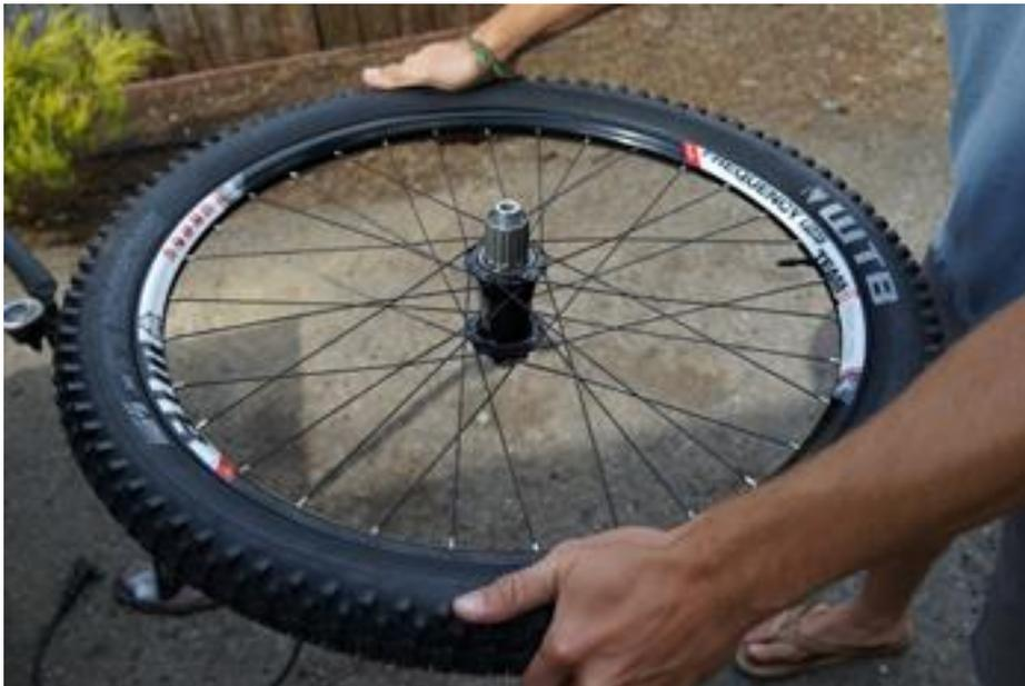
Swishing tire sealant around, gyrating the tire with both hands.
