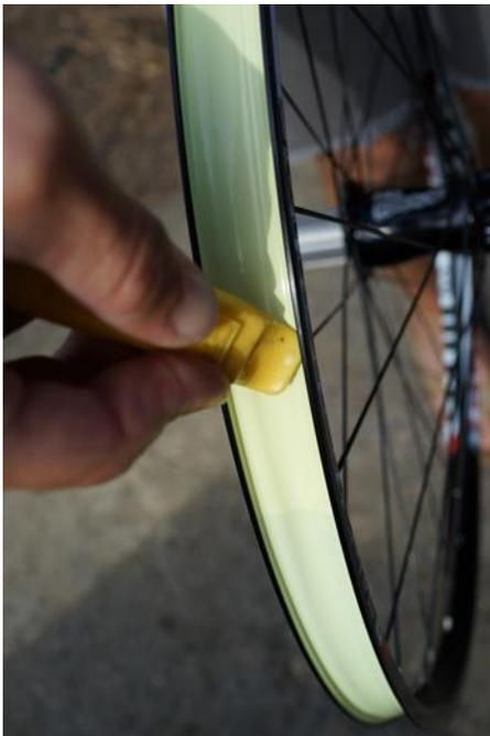
Using the smooth end of a tire lever to firmly press WTB TCS tape into place as described in Step 12
