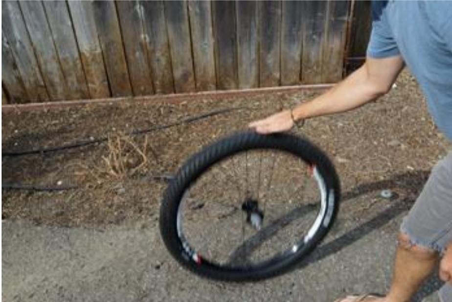
Alternative method to swishing sealant around – dribbling tire.
