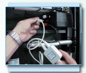
**Step 3** Connect handset remote with the pairing Cable and finish the paring.
