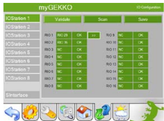
Scanning the RIO modules
