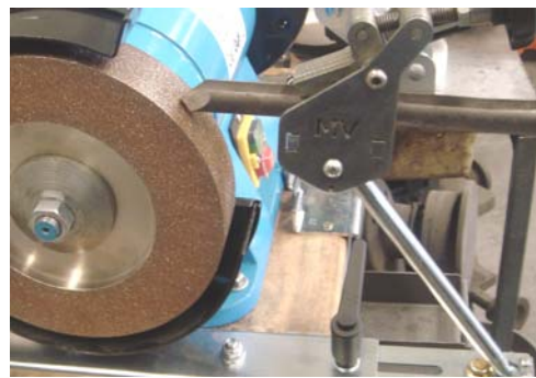
Roughing and Bowl Gouges - 44°
