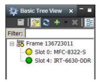
On the left the basic tree view shows the frame. With the tree structure expanded a list of cards within the frame is shown. In this example, slot position 4 is IRT-6630-DDR. When selected, all sections and tabs to the right of the basic tree view now relate to the card in slot position 4. The name of the card, in this case IRT-6630-DDR, can be set under its Configuration TAB setting.
