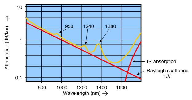
Figure 1: Attenuation versus wavelength.
