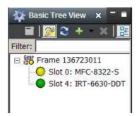
On the left the basic tree view shows the frame. With the tree structure expanded a list of cards within the frame is shown. In this example, slot position 4 is IRT-6630-DDT. When selected, all sections and tabs to the right of the basic tree view now relate to the card in slot position 4. The name of the card, in this case IRT-6630-DDT, can be set under its Configuration TAB setting.
