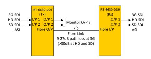
The IRT-6630-DDT and IRT-6630-DDR are transmit and receive modules designed principally for use as a serial data fibre optic transmission link for 3G-SDI, HD-SDI or SD-SDI applications conforming to SMPTE standards 424M, 292M and 259M-C using 9/125  $\mu$ m single mode fibre. This enables the use of space saving fibre optic cable for reliable transmission of digital video signals over lengths greater than can be achieved with coaxial cable.
