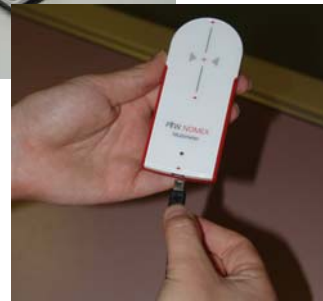
Fig. 4, 5 / USB connection to any tablet, netbook or laptop
