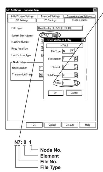
The System Area and Read Area are assigned to the PLC node designated here. Node Numbers are set via the [Mode Settings] -[Network Information] screen.
