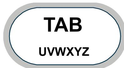
The lower margin of the push buttons contains a set of letters. For entering letters, choose the desired letter by the number of push button presses relative to the placement of that character on the push button. For example in the figure above, U is entered by pressing the **[Tab]** push button once, V is entered by pressing the **[Tab]** push button twice, etc..
