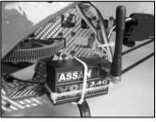
Screw out the red plastic cap on the antenna base in counterclockwise direction. Screw the 2.4GHz antenna pin into receiver base in clockwise direction. Finger tight only to avoid damage to the threads. The connecter of antenna is universal one. The antenna should point outwards during use.
