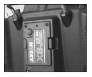
Take 2.4GHz RF model out of the package (X8F/X8J). Do not install the antenna first. Be careful not to damage the exposing part of screwing threads on antenna base.
