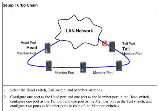
3. Connect the Head switch, Tail switch, and Member switches as shown in the diagram.
