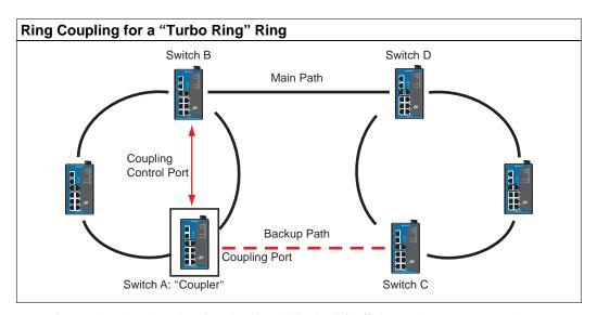
To configure the Ring Coupling function for a **"Turbo Ring"** ring, select two EDS units (e.g., Switch A and B in the above figure) in the ring, and another two EDS units in the adjacent ring (e.g., Switch C and D). Decide which two ports in each switch are appropriate to be used as coupling ports, and then link them together. Next, assign one switch (e.g., Switch A) to be the **"coupler"** and connect the coupler's coupling control port with Switch B (for this example).
