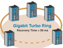
**NOTE** Port trunking and Turbo Ring can be enabled simultaneously to form a backbone. Doing so will increase the bandwidth of the backbone, and also provide redundancy. For example, suppose that two physical ports, 1 and 2, are trunked to form trunk group Trk1, and then Trk1 is set as one Turbo Ring path, if port 1 gets disconnected, the remaining trunked port, port 2, will share the traffic. If port 1 and port 2 are both disconnected, Turbo Ring will create the back up path within 300 ms.
