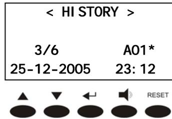
Reset of alarm A1 (MAINS FAULT) on 25/12/05 at 23:12. The position of this event in the list is the third. The total events stored in the history are six.
