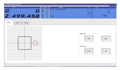
After calculating DXF files the working mold and cutter image will display on the simulation screen. The correct flow pattern will shown visually and checked.
