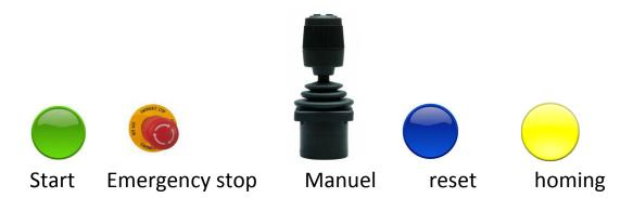
After Calculation and driver installation process the reset operation should be done, the die and cutter should be sent to reference. Emergency Stop is used to stop the machine in case of emergency. Start operation is used to run the machine after the installation process to use at mass production process.
