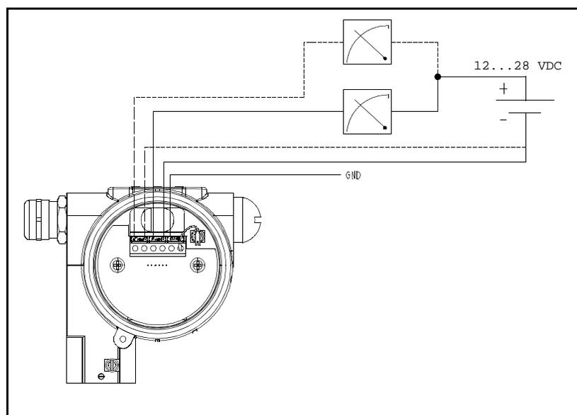
Figure 2-5: Connection with One 24 VDC Power Supply
