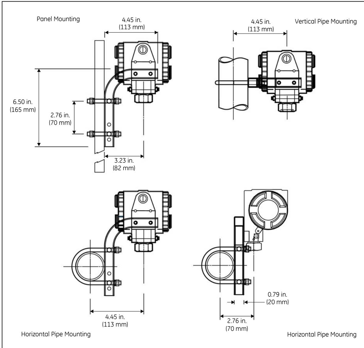
**Figure 2-2: Mounting Kit Configurations**
