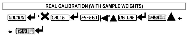
After having performed the THEORETICAL CALIBRATION and TARE WEIGHT ZERO SETTING, this function allows correct calibration to be done using sample weights of known value, if necessary, any deviations of the indicated value from the correct value to be corrected.
