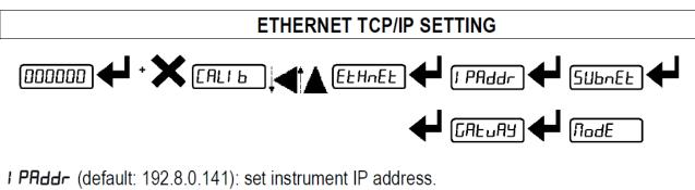
**SUB**<sub>n</sub>**EL** (default: 255.255.255.0): set instrument Subnet Mask. **GREURY** (default: 192.8.0.111): set Gateway address of Ethernet network.
