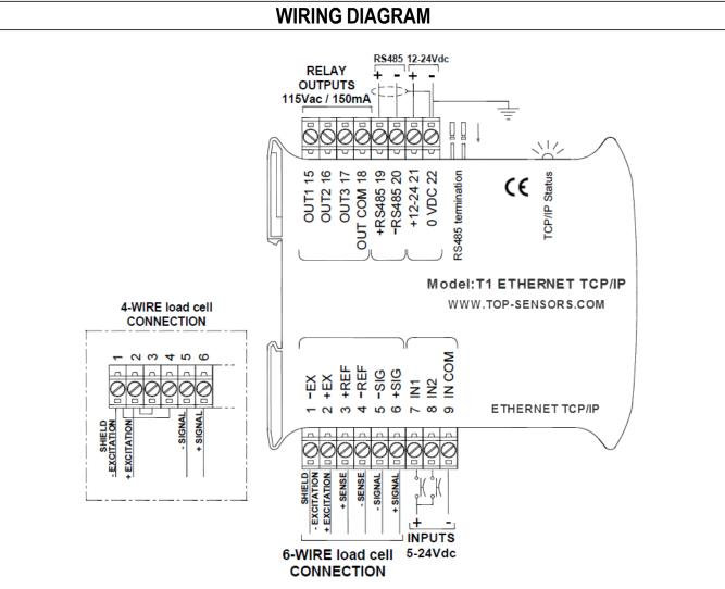
3 outputs: settable setpoints or remote output management via protocol.
