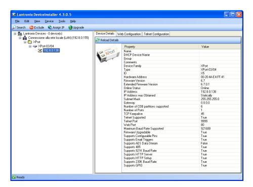
Select the found device and click on Telnet Configuration tab; click on Connect, and then press Enter on keyboard.
