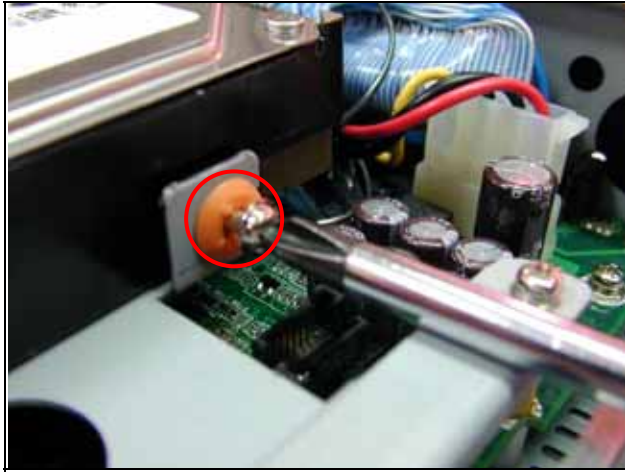
(Fig. 2-23). Fix the hard disk drive on the HDD bracket with four screws. Plug the IDE cable into hard disk drive connector
