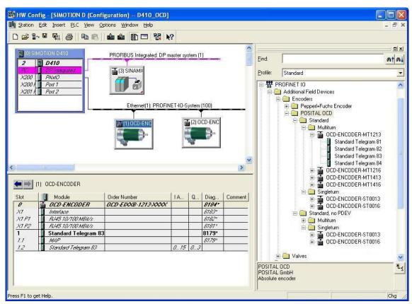
Double-click the rotary encoder icon to set communication parameters that the PLC will use. Set a device name and by clicking "Ethernet" the IP
