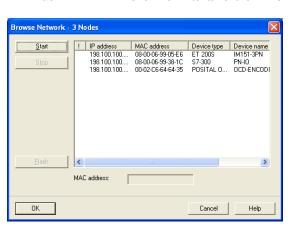
address of the chosen device to the previous window and select "Use IP parameters". The MAC address is available on the type label on the bottom left (see picture below with red marking). Enter the IP address (and subnet mask) for the encoder that you previously assigned and click "Assign IP configuration". Also, enter the device name previously chosen in the text field "Device name" and click "Assign Name".
