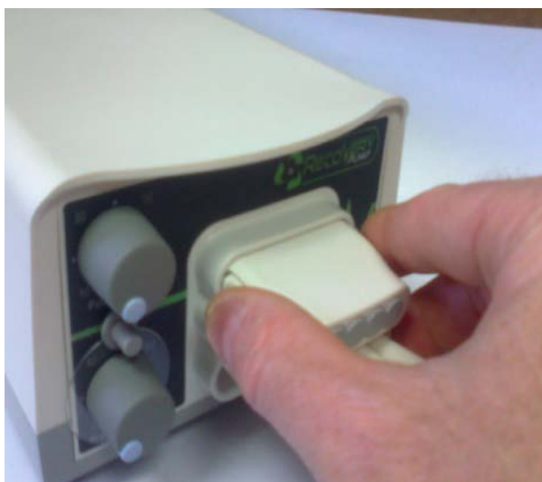
Figure 6 - Inserting the Prong Plug to Block The Unused Air Outlet for Single Garment Use
