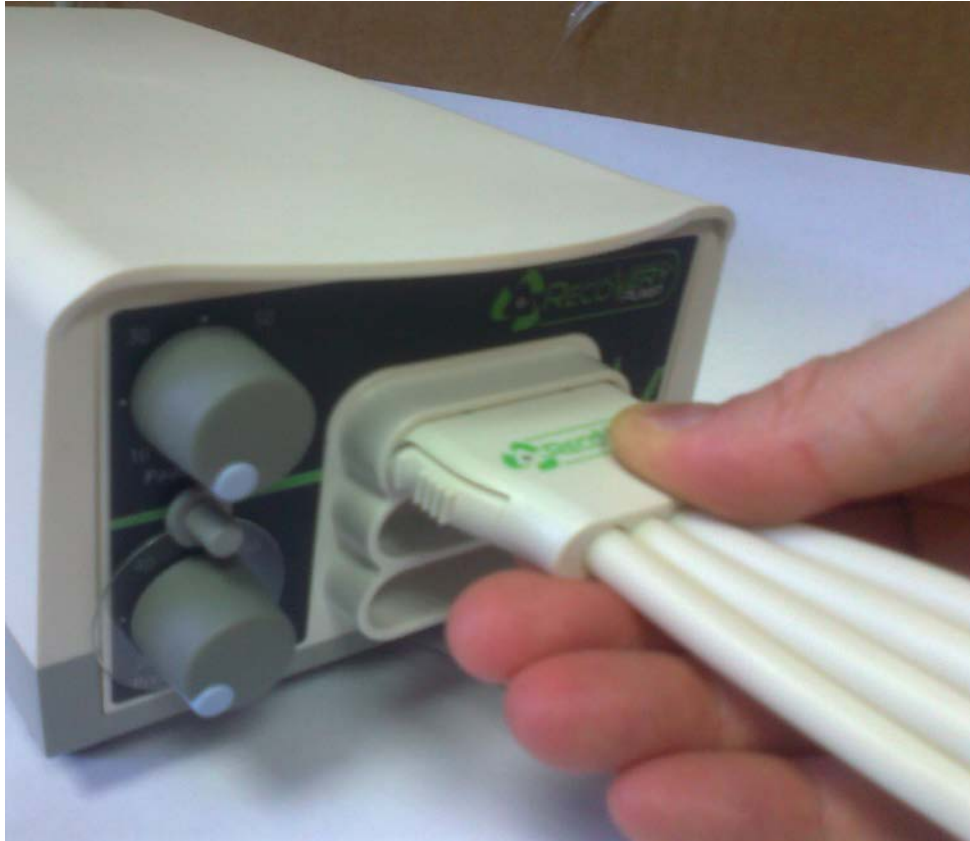
Figure 5 - Connecting the Air Hoses to the RecoveryPump™ Console
