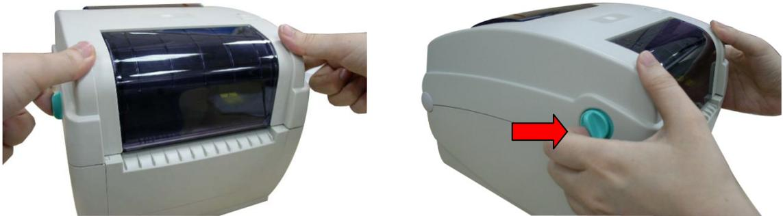
2. A top cover support at the rear of the printer will engage with lower inner cover to hold the printer top cover open.
