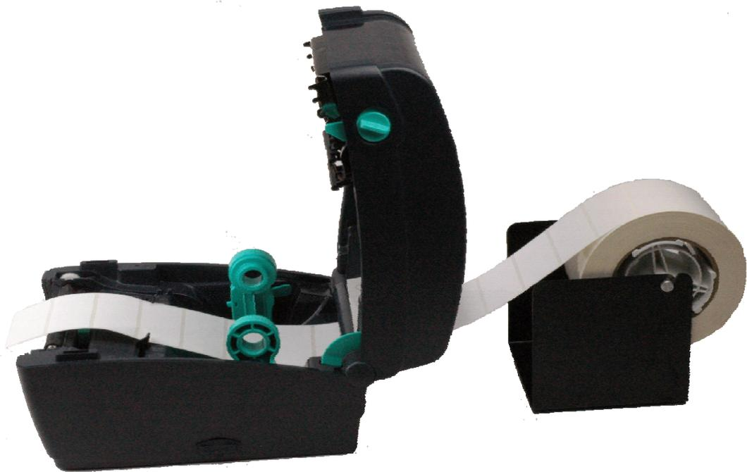
**Feed the labels as shown, close the printer securely.**
