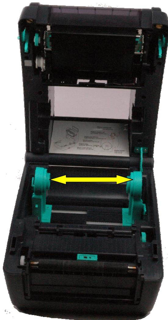
To load labels, open the TT230SM and separate the green hub guides and lock them into place on the sides. Then feed the labels from the back of the printer through the black media guides. (using the green wheel to adjust).
