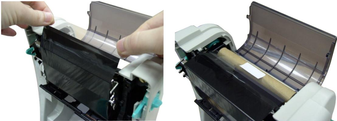
6. Turn the ribbon rewind gear until the ribbon plastic leader is thoroughly wound and the black section of the ribbon covers the print head. Close the ribbon access cover and the top cover.
