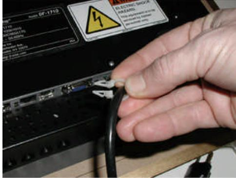
Insert the barb of the clip into one of the four 1/4" holes in the DF-1710's rear housing. These holes are slightly larger than the surrounding ventilation holes. Use one clip for landscape mode:
