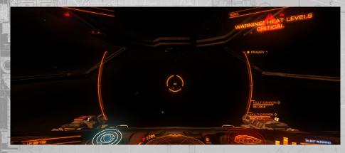
In the Pilot's Interface the ship's internal temperature is displayed as a bar directly to the left of the sensor disc.
