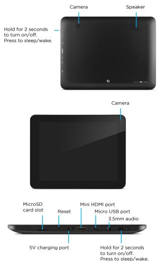
There is a small unlabeled hole on the back of the tablet. This is a button used to update the firmware. Do not press this button unless instructed to do so by Ematic.
