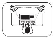
The speakers should be separated so that the tweeters form an equilateral triangle with your head. The monitors should be "toed in," or angled, so that they are pointed at you, not pointed straight ahead.
