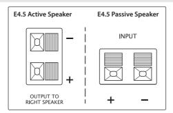
**Bare-wire connectors.** This connection is used to power and send signal to the passive E4.5. Be sure to connect the positive and negative connections on your active E4.5 to the positive and negative connections, respectively, on the passive E4.5 (i.e., connect positive to positive and negative to negative).
