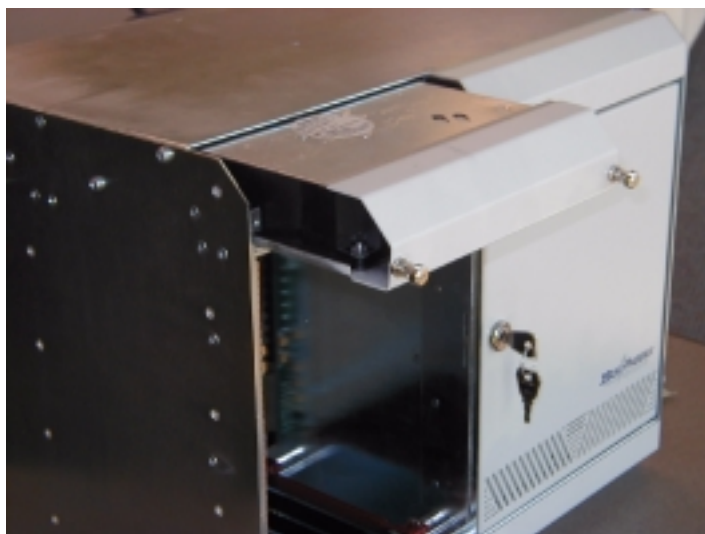
Figure 3-5: Blower Tray Partially Withdrawn
