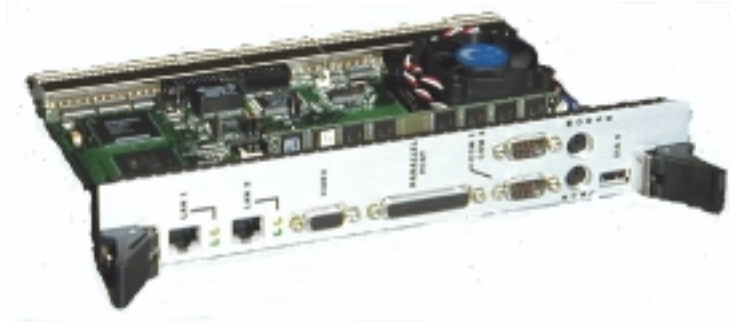
Figure 3-2: I-Bus/Phoenix IBC 2600 (Castor) CPU Board
