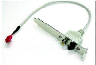
1. Connect the SPDIF output device to the rear bracket of PC, and fix it with screw.
