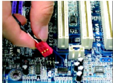
3. Connect co-axial or optical output to the SPDIF decoder.
