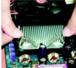
1. Fasten the heatsink supporting-base onto the CPU socket on the mainboard.
