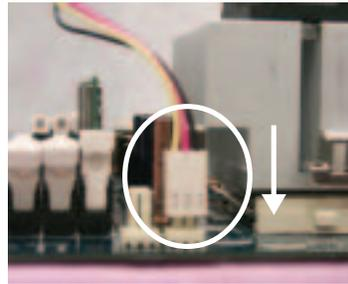
2. Make sure the CPU fan is plugged to the CPU fan connector, than install complete.
