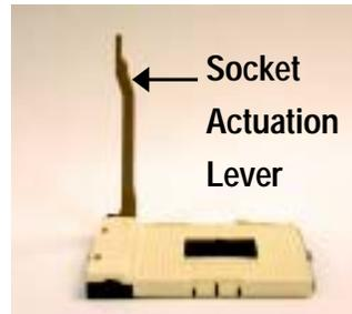
2. Pull the rod to the 90-degree directly.
