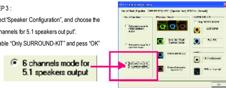
Advanced 6 Channel Analog Audio Output Mode (using Audio Combo Kit,Optional Device):
