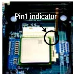
4. Locate Pin 1 in the socket and look for a (golden) cut edge on the CPU upper corner. Then insert the CPU into the socket.
