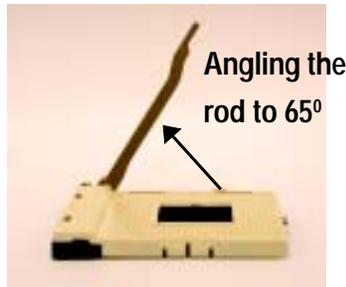
1. Angling the rod to 65-degree maybe feel a kind of tight , and then continue pull the rod to 90-degree when a noise "cough" made.
