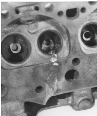
Cut Off and Peen the Plugs
