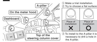
When deciding a place for installation make sure to select a place that does not interfere with airbags, standard measurement gauges, nor gets in the line of vision.
