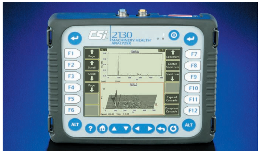
The Cascade application captures machine vibration during startup, coast-down, or over an extended period of time. Top half of screen shows spectra individually; bottom half of screen shows cascade plot.
