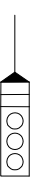
Main signal, three light units Fictive point speed information 1 and 2 associated with the main signal
