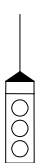
Main signal, three light units Fictive point speed information 1 associated with the main signal
